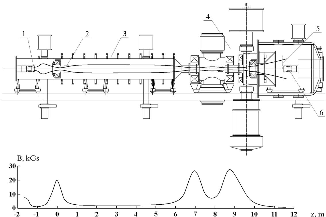
Fig.1. Side view of the magnetic system and vacuum chamber of AMBAL-M.
