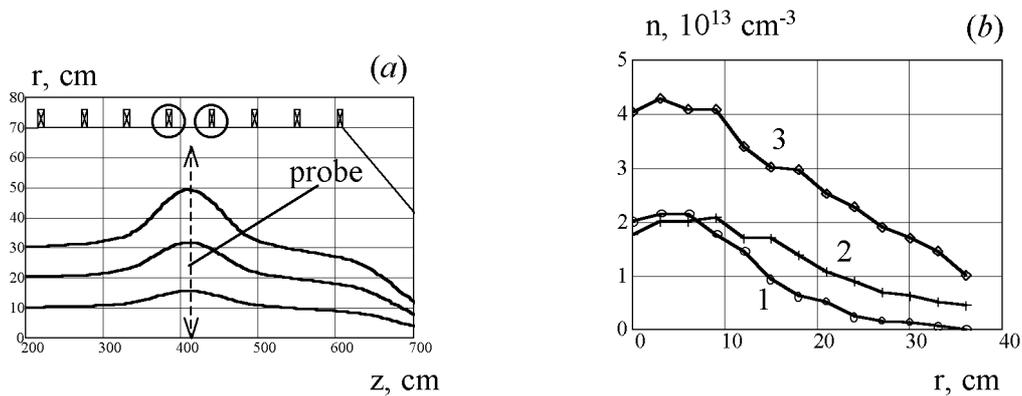
Fig.3 Schematic layout of the local mirror trap in the solenoid (a), and plasma density profiles in the middle of this trap. 1 – uniform magnetic field, 2 – with the local trap, 3 – local trap and gas puffing.
