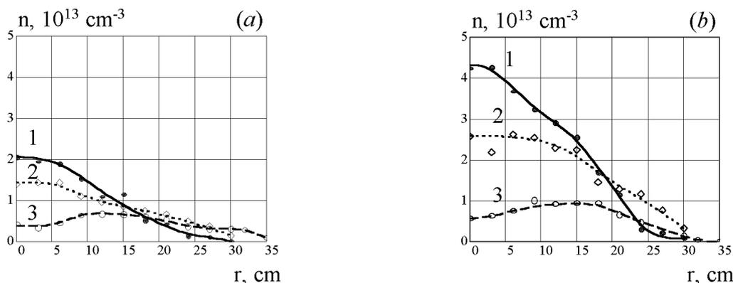
Fig.2. Radial profiles of the plasma density in the solenoid at decreased solenoid magnetic fields. *a* –without gas, *b* –with hydrogen puffing. 1 – nominal magnetic field  $B_0$ , 2 – reduced magnetic field  $B_0/2$ , 3 –  $B_0/4$ .
